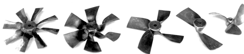
Figure 6. Experimental impellers with fixed blades. Source: [5].
