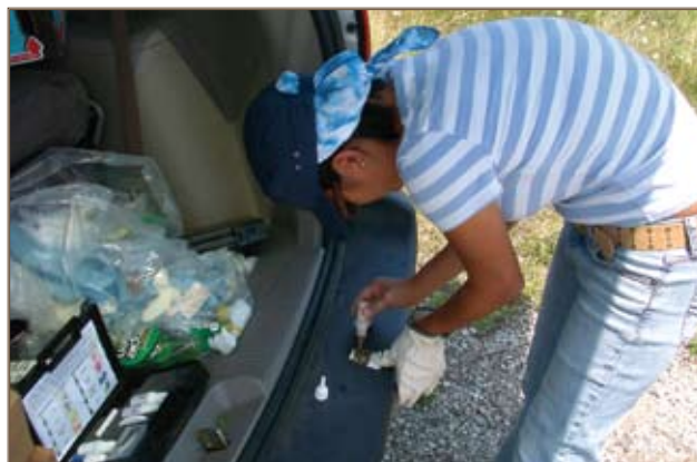
Field test technologies are often the best alternative for providing the user with a quick accurate response. Here, a field test kit is used to determine the presence of explosives in a soil sample. U.S. Army Engineer Research and Development Center photo
