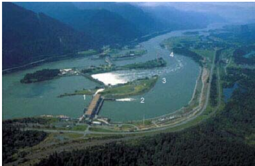
Figure 9. Bonneville Dam showing locations of the Corner Collector (1), original Corner Collector outfall (2), new Corner Collector outfall location (3) and the outfall location for the juvenile salmon turbine bypass. Photo was taken before both outfalls were extended. (Photo courtesy of U.S. Army Corps of Engineers)
