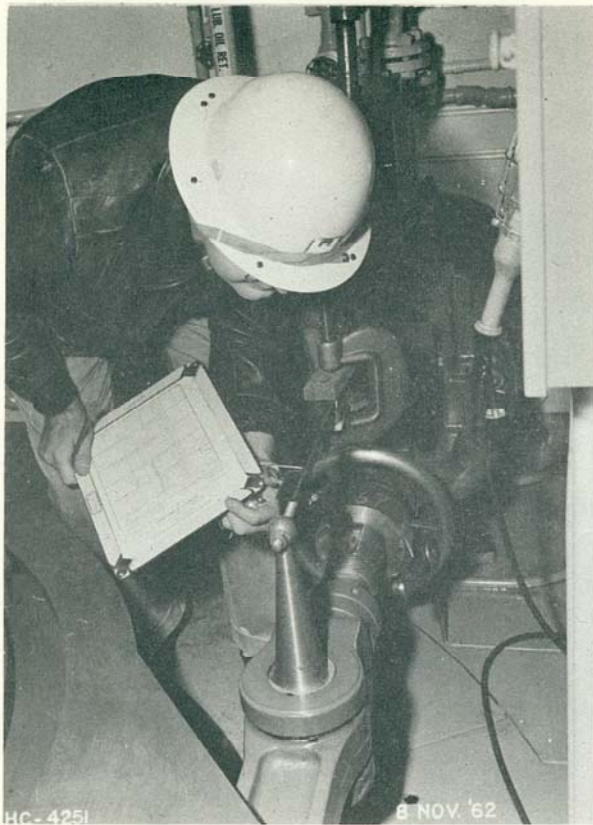
GATE SERVOMOTOR STROKE MEASUREMENT USING MACHINIST'S SCALE WITH POINTER CLAMPED TO RESTORING CABLE MECHANISM
