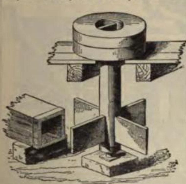
Fig. 6.—Ancient Indian Water Wheel. (After Glynn.) Containing Fundamental Suggestion of Both Turbine and Impulse Wheels.
